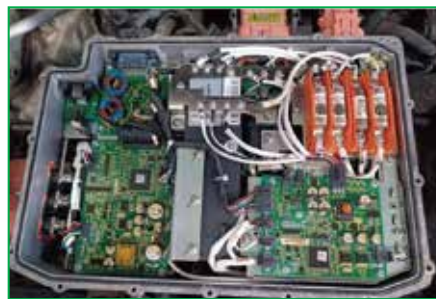
Precharge resistor, reverse diode burned out
